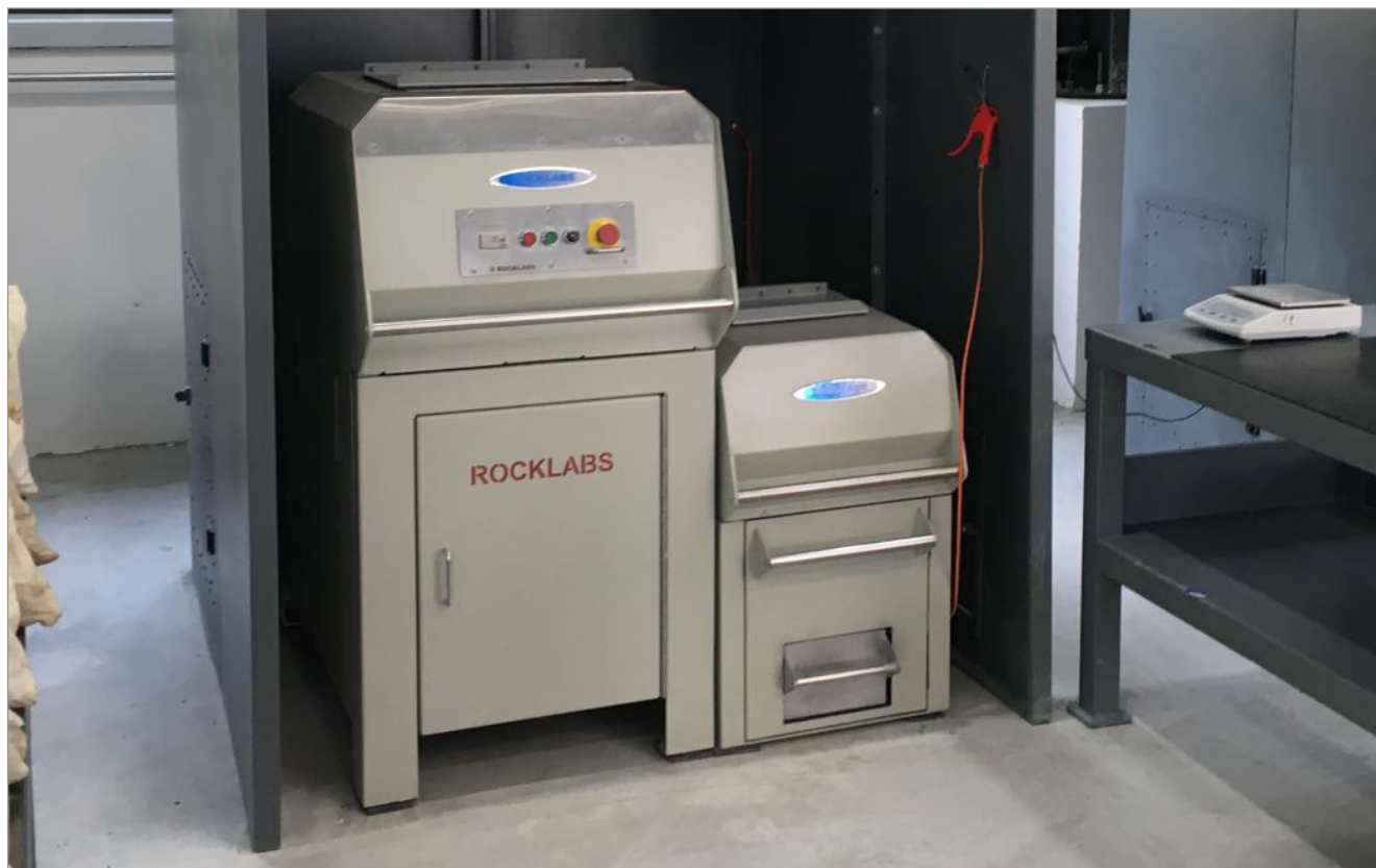
Figure 11.2 SGS Tianjin jaw crusher and RSD
