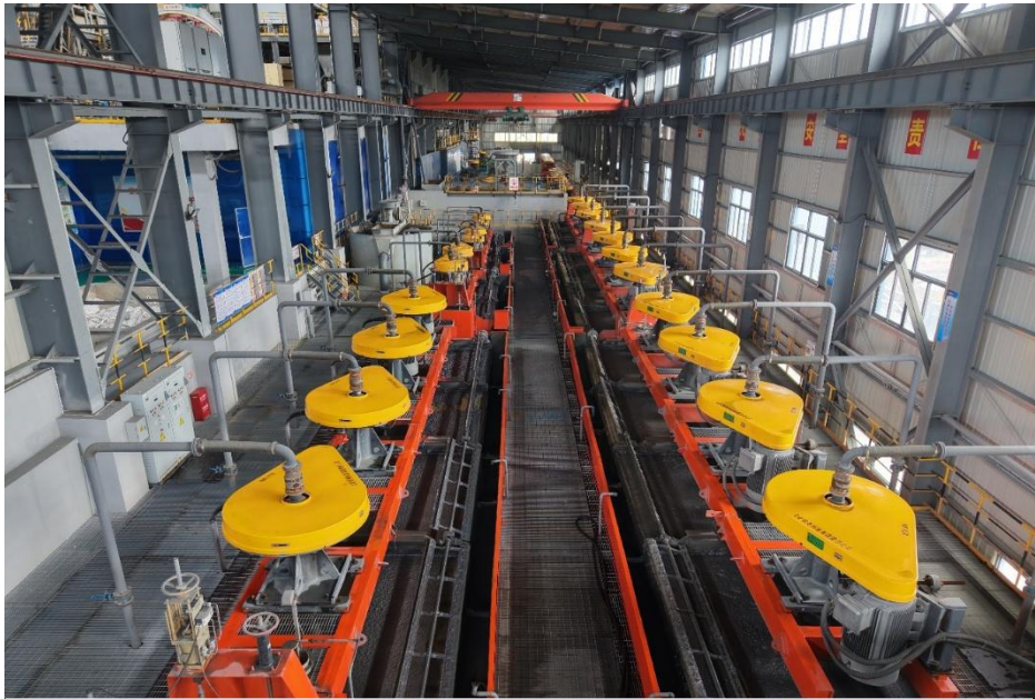
1800 TPD Flotation Line Added to Mill No. 2
