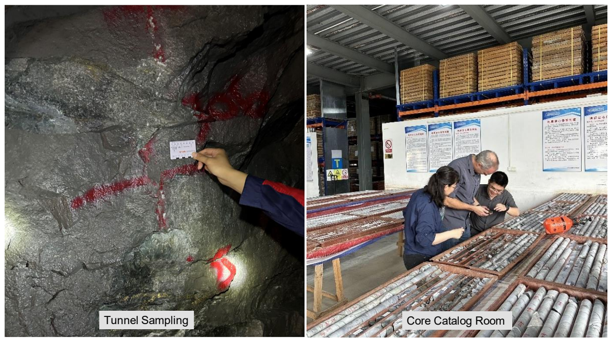
Figure 12.1: Tunnel Sampling and Core Store Shed of GC Mine
