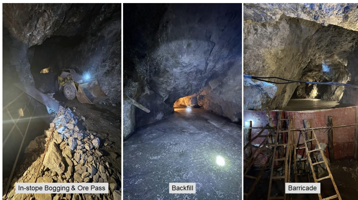
Figure 16.7: Operation of OCAF Stope
