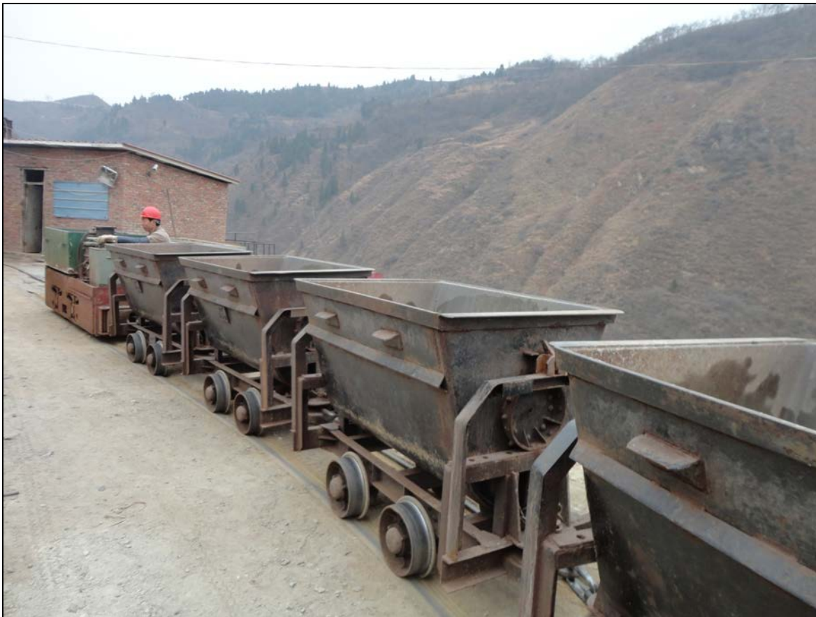
Figure 16.7 Ying loco and rail cars
