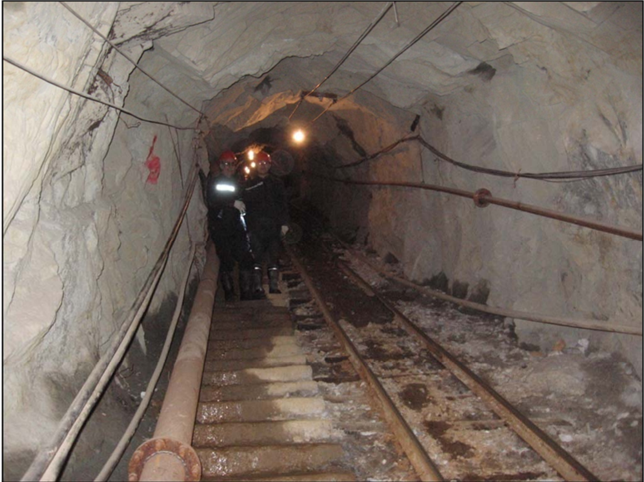
Figure 16.2 Inclined haulageway at SGX mine
