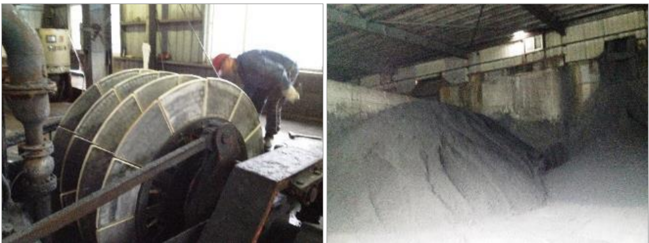
Figure 17.7 Disc filters and zinc concentrate shed
