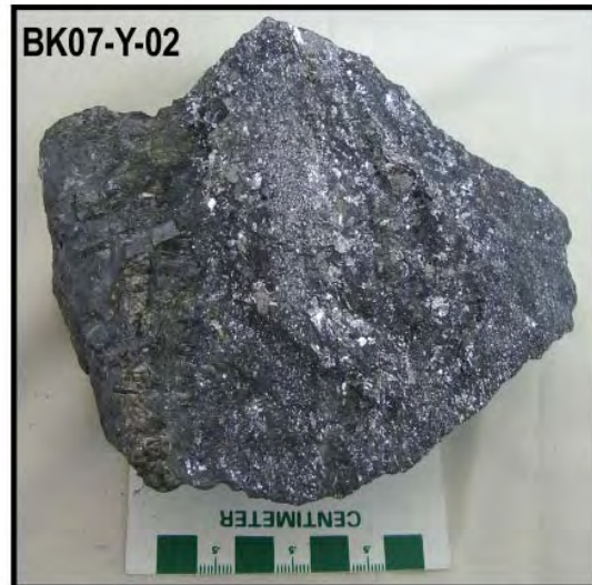
Sample BK07-Y-02, massive vein: Steel galena (dark silvery gray) with massive coarse dark sphalerite ('blackjack sphalerite', brownish-black, left-quarter side of sample).
