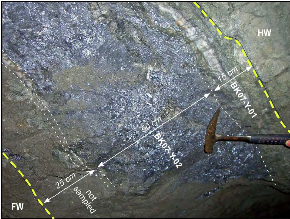
Photo of S-21 vein on level 650 of the SGX area, Ying deposit, showing samples collected during preparation of the current report. Representative closeup photos of these samples are shown below.
