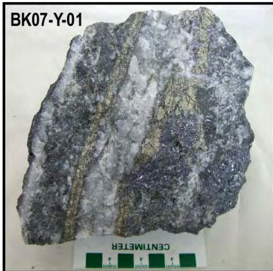
Sample BK07-Y-01, banded vein: Quartz (white), fine-grained pyrite (light yellow) and steel galena (dark silvery gray). The galena contains minor amounts of disseminated sphalerite.
